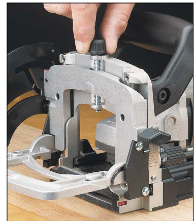
▲ A fine-threaded jackscrew for making fence height adjustments allows for extremely accurate settings.
