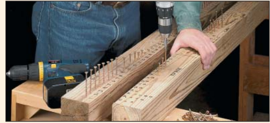
▲ We compared the clutches on the drills by driving a screw at each setting.
