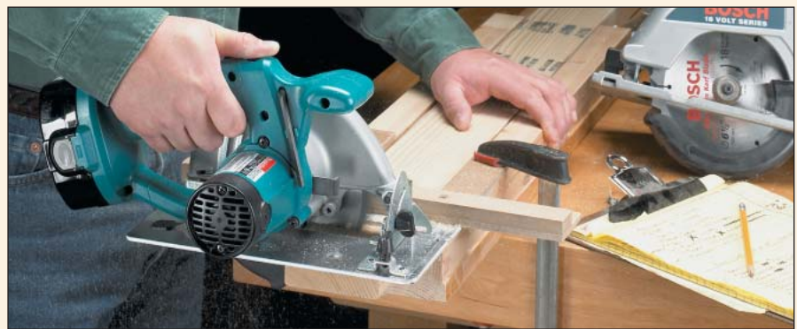
▲ The crosscut test was performed twice with each saw to ensure accurate results and allow for differences in stock. A crosscut sled guaranteed uniform cuts.
