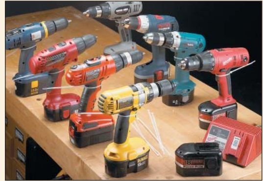
▲ The first step in testing tools is to condition the batteries. This was done by cycling each battery through five charges and five discharges.
