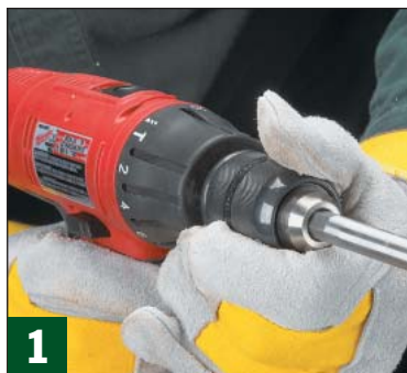
▲ The large chuck and the ratcheting action make for easy bit installation, even with gloves on.
