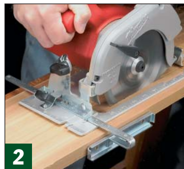
▲ The substantial fence of this edge guide keeps the Milwaukee circular saw on track during long cuts.
