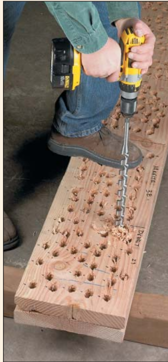
▲ To gauge the sustained power of the drills, we bored 1"-dia. holes until the batteries failed.
