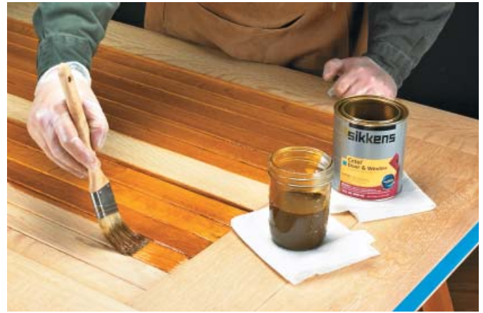
▲ To get the longest-lasting exterior finish, I chose a high-solids alkyd finish from Sikkens. It can withstand three to four years of exposure to harsh weather without needing another coat.
