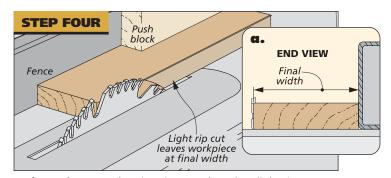
**A Clean Rip.** Once the piece is cut to length, a light rip pass on the face you cut in step one, will give you the final dimension. Any rough saw marks, burn marks, or tearout will be removed.
