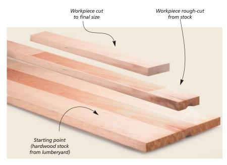
**A CUT LIST.** Before you start cutting, you need a goal. And for me, this is a cut list. I jot down a list of the parts that I need to cut and their dimensions (thickness, length, and width). Even when I'm only cutting a part or two, I write down the dimensions. It's too easy to remember a "wrong" measurement.
