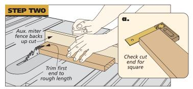
**Square One End.** Once you have two straight, parallel edges, you can begin crosscutting the workpiece to length. Start with a square, trim cut across one end of the piece.
