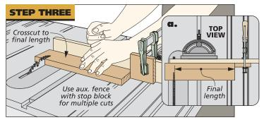
**Final Length.** A second crosscut on the opposite end gives you the final length. An auxiliary miter gauge fence with a stop block clamped to it makes multiple cuts guick and accurate.
