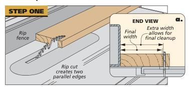
**Rip Close to Final Width.** With the straight, square edge against the fence, rip the workpiece close to its final width. The extra width allows you to clean up this face with the final cut.
