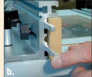
For jointing, two aluminum bars are used to shim the Bench Dog fence.
