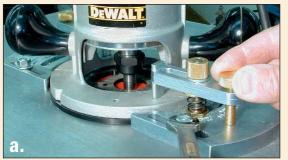
A unique, quick-clamp mechanism on the Veritas router table lets you mount or remove the router in seconds.
