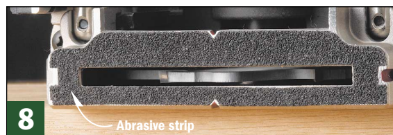
◀ Porter-Cable’s abrasive strip provides a passable grip on any size workpiece.
