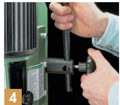
▲ With only two positions to choose from, this lever often isn't set at an optimum position.
