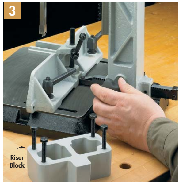
▲ The micro-adjustable fence and tool-free settings make setup fast, accurate, and secure. Installing the riser block gives this machine the largest throat capacity in the bunch.
