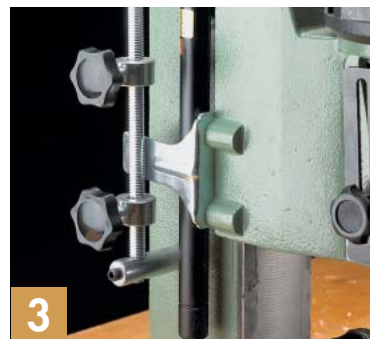
▲ General's unique stop system allows you to customize the stroke length to the job.
