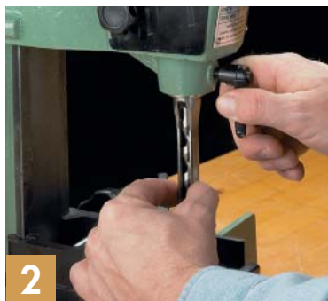
▲ The General is the only machine in the bunch with a tool-free chisel lock.
