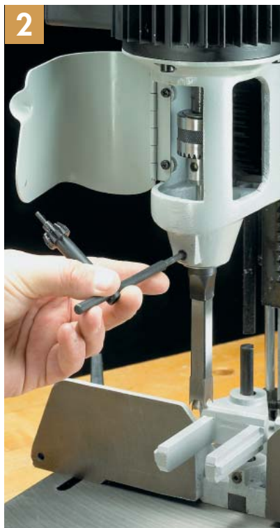
▲ The micro-adjustable fence and tool-free settings make setup fast, accurate, and secure. Installing the riser block gives this machine the largest throat capacity in the bunch.
