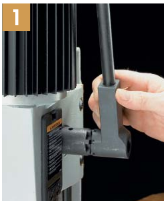
▲ Delta's 14-651 has all the best features, including a pinion-type lever that adjusts quickly and without tools.
