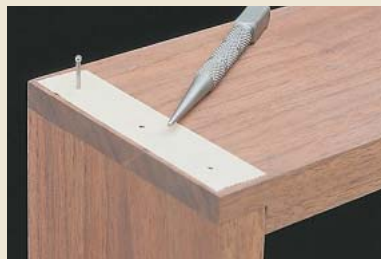
▲ Before picking up the hammer and nails, first apply a strip of masking tape. Then drive and set the nails.
