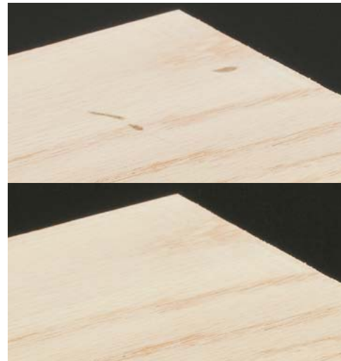
▲ With a little steam from a hot iron (see photo at left), the compressed fibers of a dent will swell back into place.
