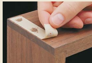
▲ Now force putty into the holes and remove the tape. The small "bump" that remains can be sanded away.
