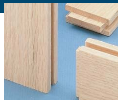
▲ Stub tenons, like those shown above, are often used in the construction of frame and panel doors.
